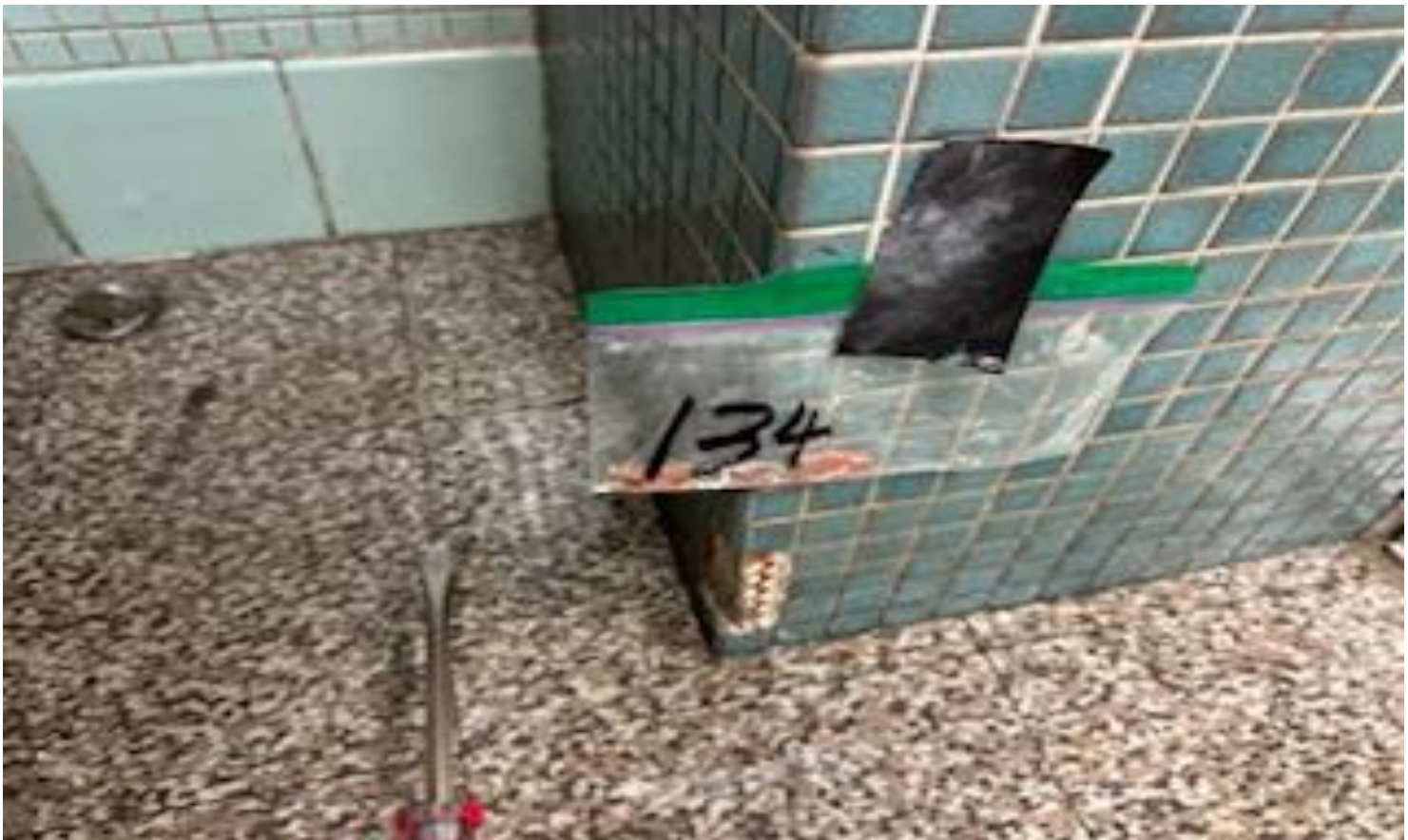
60. VIEW OF REPRESENTATIVE (TYPICAL) SAMPLE OF NON-ACM GREEN COLUMN WALL CERAMIC TILES AND GROUT LOCATED THROUGHOUT THE BUILDINGS AT THOMAS C. MARSH PREPARATORY ACADEMY
