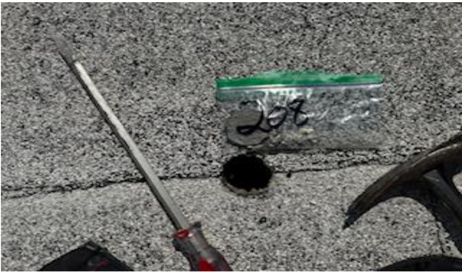
81. VIEW OF MORE REPRESENTATIVE (TYPICAL) SAMPLE OF NON-ACM ROOF CORE PROFILE SAMPLE LOCATED THROUGHOUT TOP ROOFS OF THE BUILDINGS AT THOMAS C. MARSH PREPARATORY ACADEMY
