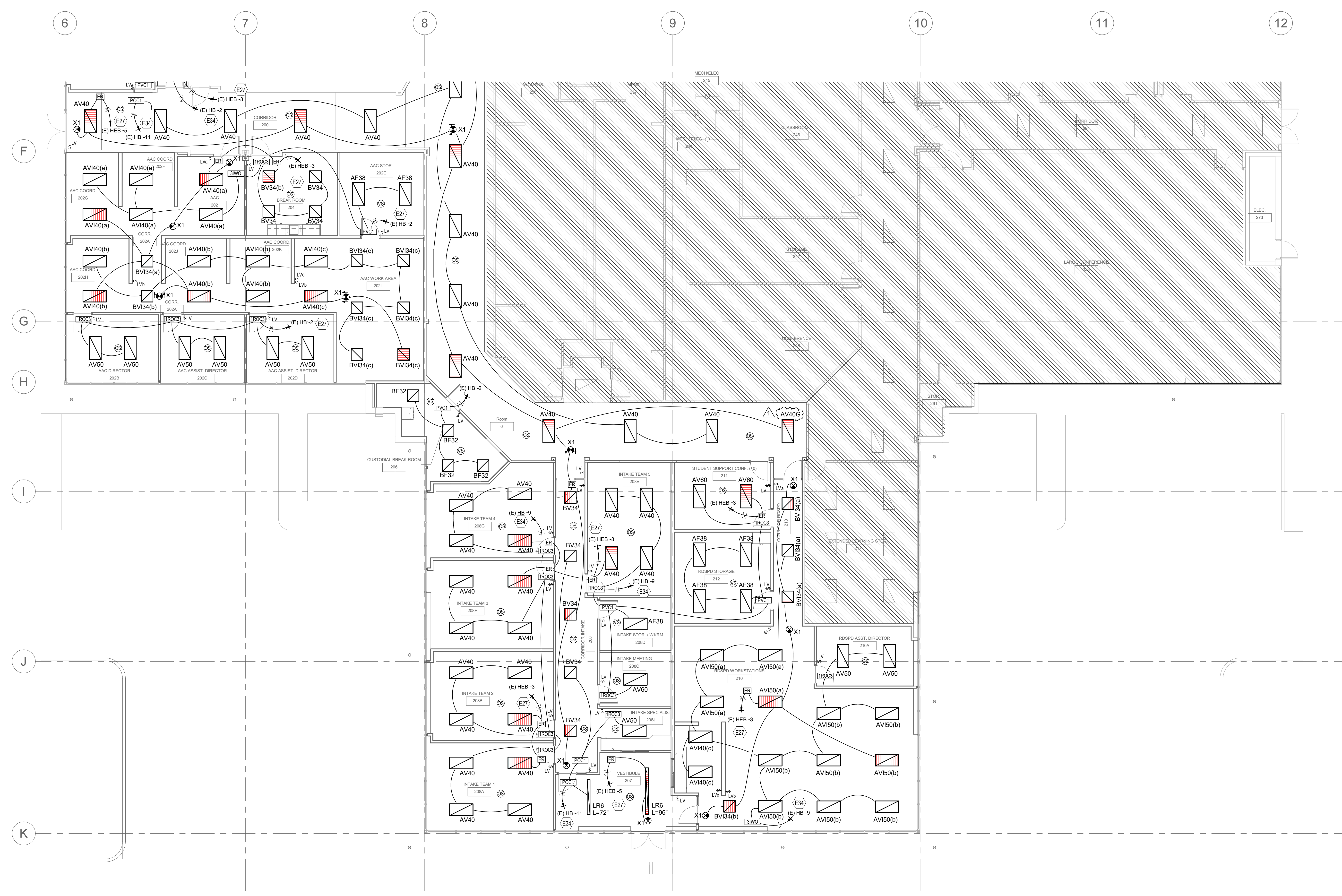
1 LEVEL 01 LIGHTING PLAN - BUILDING 2S 1/8" = 1'-0"
